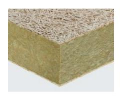
Composite thermal and acoustic insulation board, in Euroclass A2-s1, d0, consisting of two layers (thickness 5 mm each) of mineralized thin fir wood wool bound with white Portland cement and mineral powder, coupled to an internal layer of high density mineral wool according to EN 13162 standard. Wood wool is 2 mm wide. It complies with EN 13168 standard.
