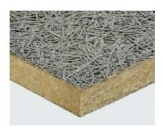
Composite thermal and acoustic insulation board, consisting of two layers (thickness 5 mm each) of mineralized fir wood wool bound with grey Portland cement coupled to an internal layer of high density mineral wool according to EN 13162 standard. It complies with EN 13168 standard. CELENIT L3 is PEFC™ certified. Also available with FSC® certification.
